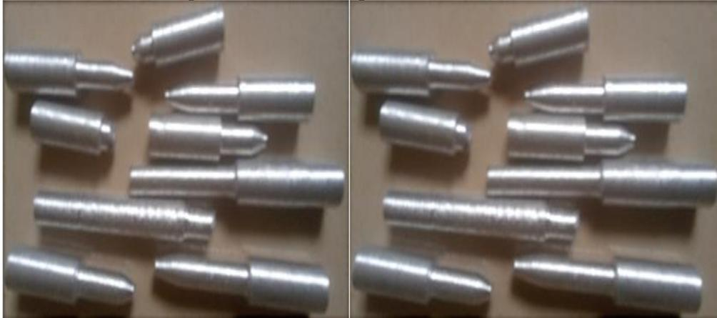
**Figure 9: Fractured test samples after tensile test**
